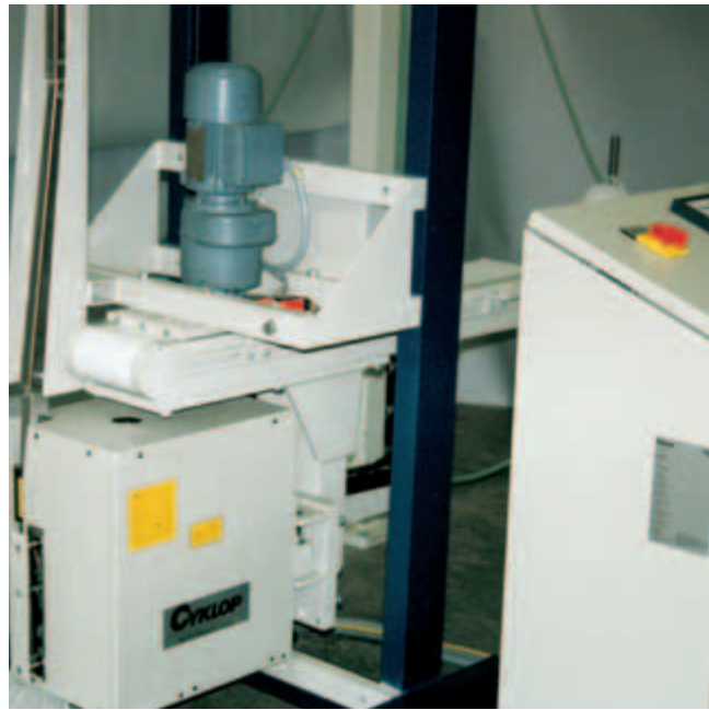
Picture 8. Head travel device with drive. Control desk
